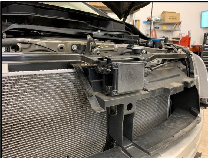
*Honda Accord Millimeter Wave Radar*
