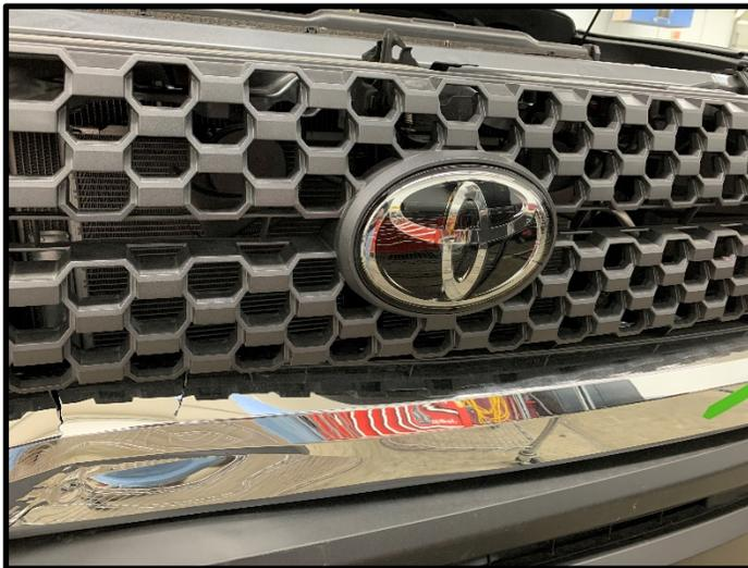
Millimeter Wave Sensor behind Toyota Emblem
