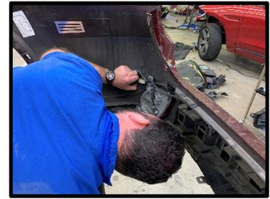
Installation of Ultrasonic sensor, rear bumper
